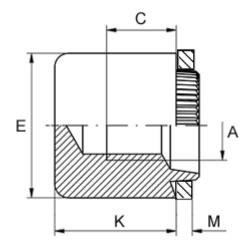
Female thread A = M12Height K = 19.0Min thread length C = 7.0Outer diameter E = 25.0Plate thickness = 3.2 to 3.4
